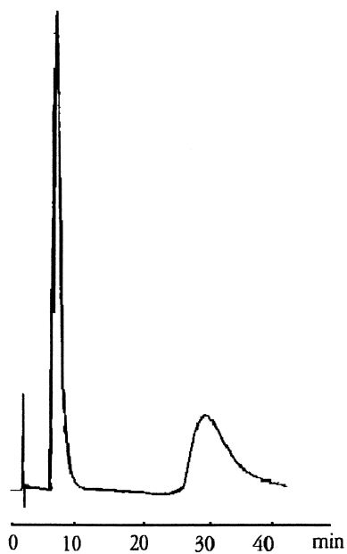
Figure 5. Compound No.3; mobile phase, n-hexane: 2-propanol (93:7), temperature 20°C, on cellulose tris(3,5-dimethylphenyl carbamate) CSP.
